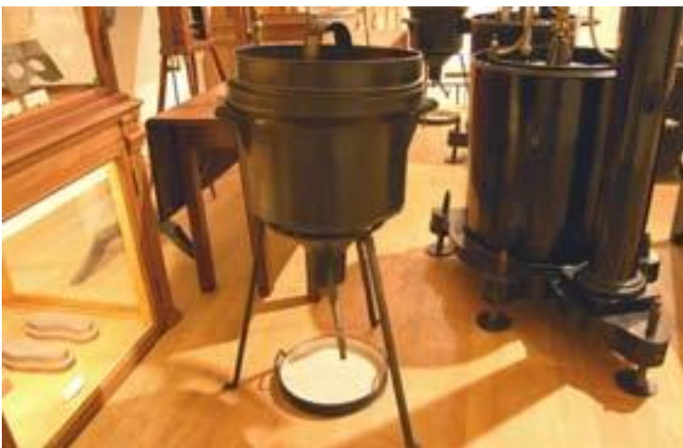
Figure 7. The 'calorimeter' used in the guinea pig experiments
